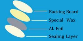
★ Flexible WAD, recently market of this wad grown up due to Easy Peelability and Pull Tab to ease the opening of sealing of PP Jar.
